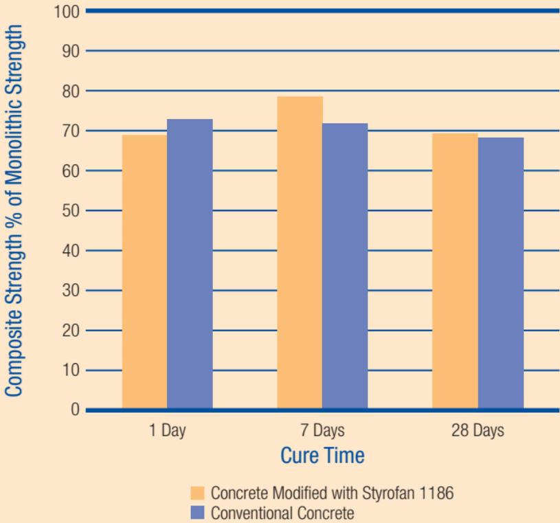
1. Composite psi is the compressive force to fail the composite cylinder
